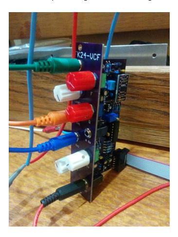
The module is designed and sized for **Eurorack** systems. You will need a 16-10 pin **Eurorack** power ribbon connector with -12/0/+12 which is connected to a synth power supply. You will also need a trimmer adjustment tool, a digital volt meter, a frequency counter and, if possible, an oscilloscope.
