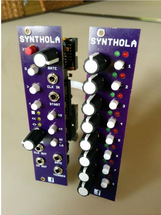
The module is designed and sized for **Euro rack** systems. You will need a 16-pin **Euro rack** power ribbon connector with  $-12/0/+12$  and  $+5V$  which is connected to a synth power supply.
