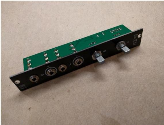
3. Now fully solder as many of the remaining pins on the jacks and pots that you can access without burning nearby components.
