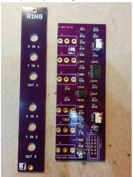
The module is designed and sized for **Eurorack** systems. You will need a 16-10 pin eurorack power ribbon connector with -12/0/+12 which is connected to a synth power supply.
