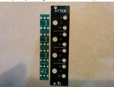
The module is designed and sized for **Eurorack** systems. No power supply is needed for this module. Follow the parts lists, these instructions and the PCB silkscreen text to build the module. Please ensure that you place the components on the correct side. There are components installed on BOTH SIDES of the board.
