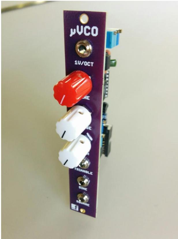
The module is designed and sized for **Euro rack** systems. You will need a 16 pin **Euro rack** power ribbon connector with  $-12/0/+12$  which is connected to a synth power supply. You will also need a trimmer adjustment tool, a digital volt meter, a frequency counter and, if possible, an oscilloscope.
